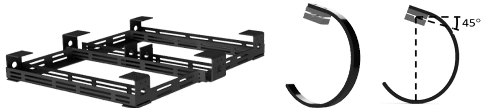
Fig. 2. Image (a) showing the designed RHex frame without the top and bottom plates. Image (b) showing the C-Shaped compliant leg with motor coupler.
